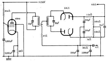
Circuit values used in ratio detector described by Seeley and Avins (RCA Fig. 16. Review, June 1947).
