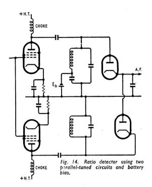
a.m. handling capacity is proportional to the amount by which the input signal exceeds the "threshold" input required by the limiter. In the ratio detector, the maximum "downward" a.m. handling capacity is a fixed quantity. In general a detector should be capable of handling "downward" modulation of the order of 50 per cent, and both circuits can normally achieve this.
