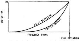
Fig. 13. Showing how distortion varies for ratio detector and Foster-Seeley circuits having equal distortion at full deviation.
